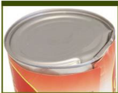
Severe dent in seam
